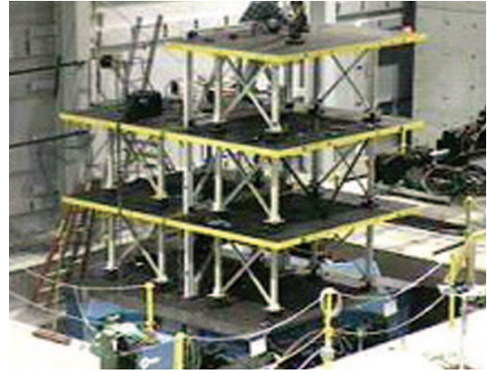
Shake table test of steel structure with advanced braces (zipper frames)
