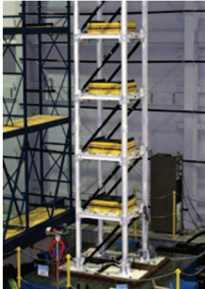
Testing of added clamping system in 5-story structure
